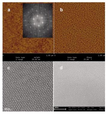
Fig 2. AFM height (a) and phase (b) images  $(1 \ \mu m \times 1 \ \mu m)$  of the thin film. Inset shows the corresponding Fourier transform. TEM (c, scale bar = 100 nm) and SEM (d, scale bar = 300 nm) images of the thin film after removal of the PEG cylinders.
