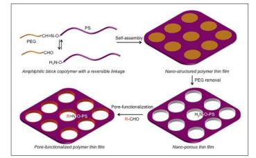
Fig. 1. Schematic representation of nanostructured thin film formation from self-assembly of dynamic covalent diblock copolymer, subsequent step of pore formation due to the reversibility of the copolymer linkage, and tentative graphic representation of the functionalized-pore.
