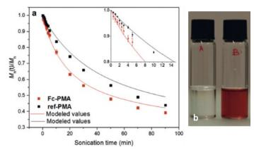
Fig. 2 a) Decrease of the normalized molecular weight  $(M_n(t)/M_n)$  of ref-PMA (black) and Fc-PMA (red) as a function of sonication time in THF. b) Pictures showing a Fc-PMA solution to which KSCN had been added before (left) and after (right) sonication. The red Fe-thiocyanate complex formed after sonication confirms the release of Fe ions upon sonication. Copyright (2018) Angewandte Chemie International Edition.
