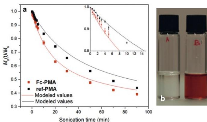
Fig. 2 a) Decrease of the normalized molecular weight ( $M_n(t)/M_n$ ) of ref-PMA (black) and Fc-PMA (red) as a function of sonication time in THF. b) Pictures showing a Fc-PMA solution to which KSCN had been added before (left) and after (right) sonication. The red Fe-thiocyanate complex formed after sonication confirms the release of Fe ions upon sonication. Copyright (2018) Angewandte Chemie International Edition.
