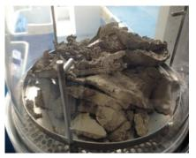
Suspended matter collected with the centrifuge at the international monitoring station Weil am Rhein. Collecting time depends on the turbidity of the river water, typically, it is 24–48 h (photo by R. Dolf).
