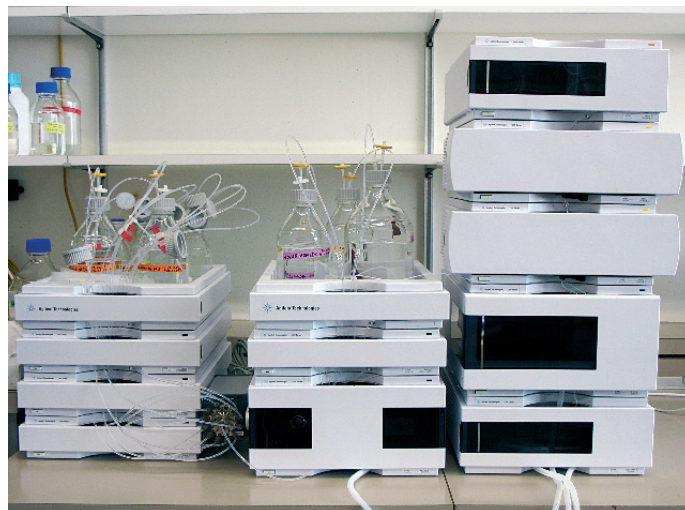
HPLC method development platform with high pressure option up to 600 bar.
