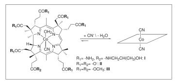
Structural formula of the corrin-based chemosensors I-III and a schematic representation of cyanide detection (right).
