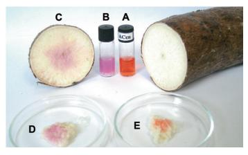
The orange corrin-based chemosensor (A) turns violet in the presence of cyanide, as in an aqueous solution of crude cassava (B), a freshly sliced cassava surface (C) or a ground cassava extract (D). No cyanide is detected after thorough washing of the ground cassava extract (E).
