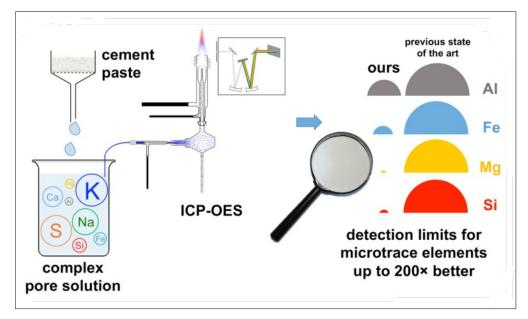
The proposed ICP-OES method allows the simultaneous, very accurate determination of high- (Ca, K, Na, S) and low-concentration (AI, Fe, Mg, Si) elements of the pore solutions from cement pastes, with and without superplasticizers.
