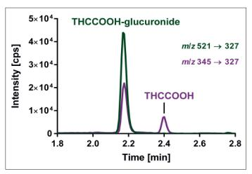
Chromatogram of an authentic whole blood specimen from a cannabis consumer (THCCOOH, 97.6  $\mu$ g/L); THCCOOH-glucuronide, 296  $\mu$ g/L). The purple peak at 2.16 min corresponds to the THCCOOH fragment originating from in-source decay of the glucuronide.
