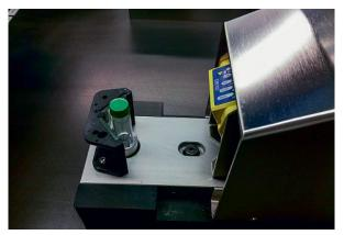
Fig. 2. Barcode reading, weighing, and photo documentation.
