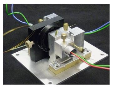
The detector cell for capillary electrophoresis.
