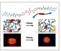
formation of a dynamic supramolecular polymer. The new material exhibits the characteristic thermomechanical properties of a supramolecular polymer, offers three different emission colors in the solid state and exhibits both mechano- and thermoresponsive luminescence.
