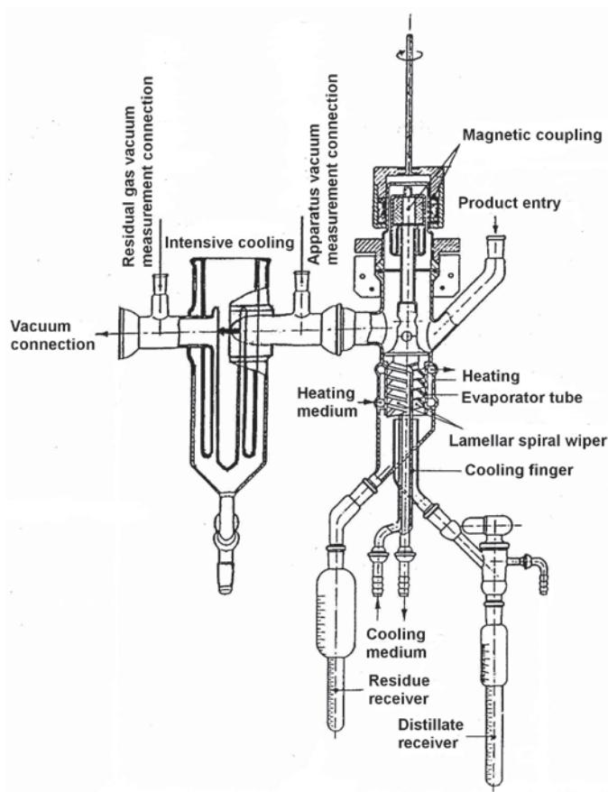
With the all glass exterior evaporator with the innovative flat profile lamellar spiral wiper which is in use in distillation, research and development laboratories, thermolabile or high-molecular substances can be distilled with approximately 5 to 10 seconds exposure time and minimal temperature at atmospheric pressure to high vacuum. As the substance gets only in contact with borosilicate glass all over the apparatus, the often observed catalytic decomposition on metal surfaces of
