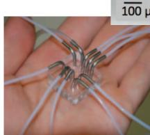
Photograph of a microdevice made of poly(dimethylsiloxane), channel inlets and outlets are connected to tubings.
