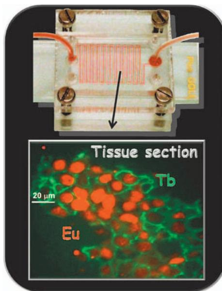
Microfluidic device and its potential for dual assays: ER (red) and Her2/*neu* (green) receptors evidenced by time-resolved luminescence microscopy. Her2/*neu* receptors: polyclonal rabbit anti-human c-erbB-2 oncoprotein antibody / Tb-labelled goat anti-rabbit IgG antibody. ER receptors: anti-human ER mouse mAb / Eu-labelled goat anti-mouse IgG Ab.
