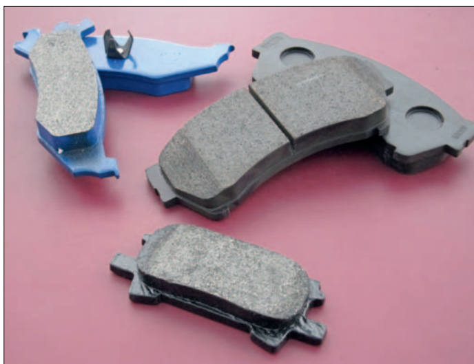
Brake pads with their temperature-resistant, hard linings composed from binder materials and heavy metals, some of them toxic.
