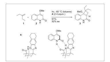
Prof. Thorsten Bach showed how to control the enantioselectivity in photochemical reactions by using the chiral template **4** and its coordination with the substrate **2** (*J. Am. Chem. Soc.* **2000**, *122*, 11525).
