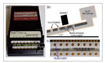
a) GRAVI™-Cell device with an 8-microchannel chip tilted at 30°. b) Cross-section along the microchip showing magnetic beads trapping. c) GRAVI™-Chip comprising 8 microchannels, inlet reservoirs at the top and outlet ones at the bottom.
