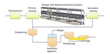
Flow chart of a typical plant: The 1000-litre microbial fuel cell: its function in a typical wastewater treatment plant (Photo: HES-SO Valais).
