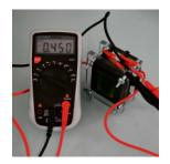
Small scale microbial fuel cell with multimeter, assembled by the participants in the workshop of Professor Fabian Fischer and used in experimental work. Photo Marc Sugnaux, HES-SO Valais.
