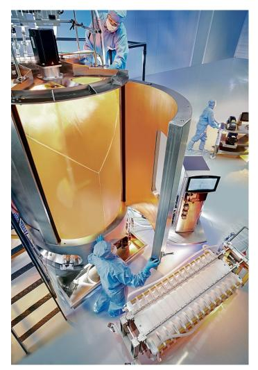
The BIOSTAT® STR of Sartorius offers true scalability in single use and is ideal for high density cell culture applications, monoclonal antibody, recombinant protein and vaccine production as well as seed cultivation for large-scale bioreactors. (Source Sartorius Stedim)
