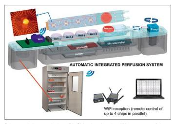
Scheme of the stand-alone BioChip showing the different parts of the integrated system. A miniature peristaltic pump allows the perfusion of the culture medium from the reservoir to the different wells through a Bluetooth remote control. The insert shows a 3D neural culture derived from hESCs placed onto the multi-electrode array. Recordings of electrical signals are sent to the acquisition software through a WiFi transmission. Image: Luc Stoppini.
