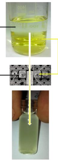
Fig. 2. Poorly miscible native oil and alcohol (top) can be mixed appropriately using microreactor technology.
