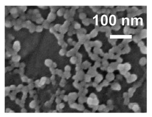
Fig. 5. Scanning electron micrograph of nanoparticles from continuous crystallization in a microreactor system.
