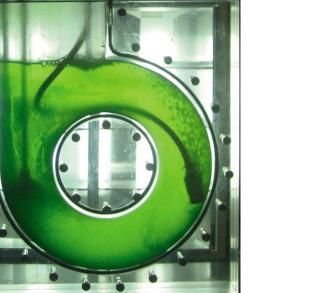
Fig. 3. Torus photobioreactor with micro algae cultivation.
