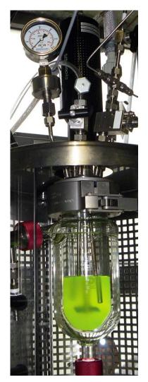
Fig. 1. Hydrogenation reactor.
