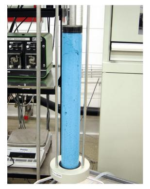
Fig. 4. Cu<sup>2+</sup> adsorption on a fixed bed of chitosan microbeads.
