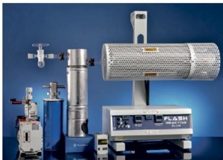
(vacuum) the number of collisions between the molecules is low. Moreover, the vacuum increases the speed of migration of particles through the reactor zone resulting in short residence times (typically in the millisecond range). These properties collectively minimize the chance for side-product formation.
