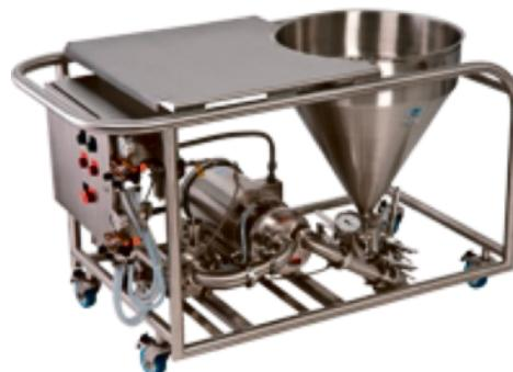
“The Fastfeed consumes up to 70% less energy than conventional tank mixers and batch-to-batch inconsistencies are eliminated as powders are introduced at the same rate every time,” notes Earley. Batch times and air entrainment are also reduced because powders. Dust from dumping powders into open top tanks is also eliminated. Operator safety is also enhanced as powders are added from the safety of floor level.
