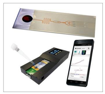
A microfluidic chip having patterned electrodes can be inserted on a small, low-cost peripheral for monitoring flow and reading assay results. Such a peripheral has a Bluetooth module, a microcontroller, and can communicate with a smartphone. This technology is broadly applicable to any ligand-receptor type of assay for the generation and analysis of precise data.
