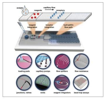
Immunoassays are implemented in capillary-driven microfluidic chips by defining a hydrophilic flow path through which a sample passes, dissolves detection antibodies, and forms an antigen-antibody complex on downstream capture antibodies. The flow path is modular and can be created using various assortments of microfluidic functional elements.
