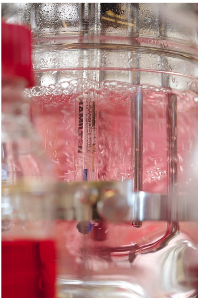
Standard stirred bioreactor at laboratory scale, prepared for the cultivation of mammalian cells, running a sterility test. Photo by ZHAW Wädenswil.
