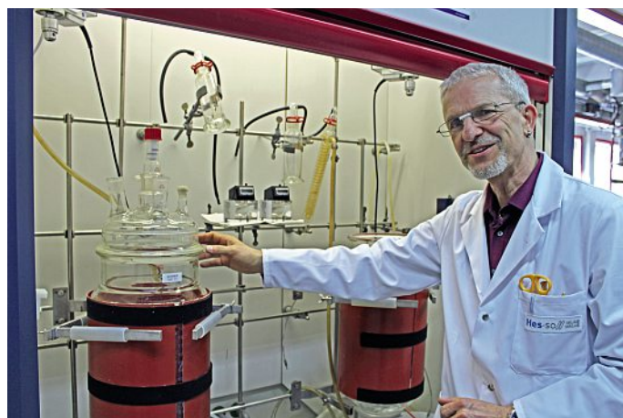
UAS professor Simon Crelier, who teaches downstream processing and enzyme technology, presents the 20-litre stirred glass reactors with temperature control for anaerobic digestion at the Biotechnology Unit of the Life Technologies Department. Photo: Elsbeth Heinzemann.
