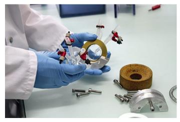
The microbial fuel cell made of glass serves in this project for experiments under sterile conditions. Photo Elsbeth Heinzelmann.
