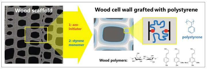
Wood cell wall grafted with polystyrene. Image ETHZ
