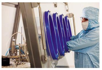
Upstream processing suite at the National Institute for Bioprocessing Research & Training (NIBRT) in Dublin, showing a completely controlled 150-litre perfusion bioreactor. (Copyright NIBRT)
