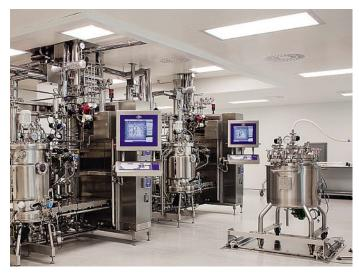
Upstream processing suite at the National Institute for Bioprocessing Research & Training (NIBRT) in Dublin, showing two completely controlled 150-litre perfusion bioreactors (left of image) and harvest vessel (on right of image). (Copyright NIBRT)
